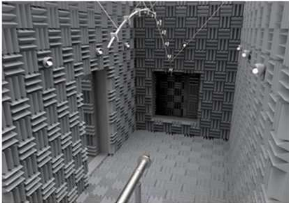
Figure 4: Rig Test chamber with acoustic treatment and microphone arc for polar angle farfield measurements
