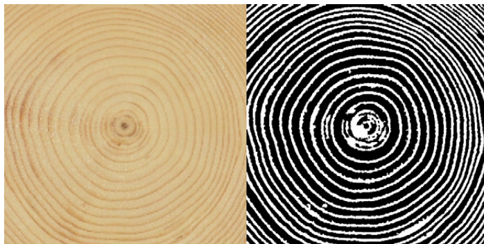
Figure 1: Sectional RGB image of log end face (left), binary image displaying segmented annual rings (right).
