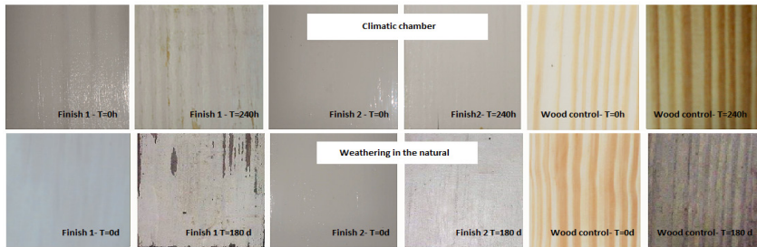
Figure 1: Colour changes of wood of Pinus sp. exposed to two weathering treatments. Two finishes are compared with control specimens.
