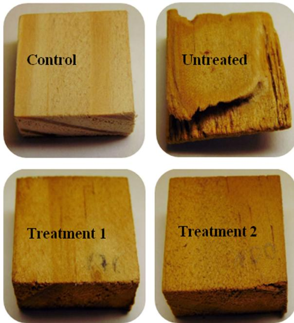
**Fig. 1** Biological attack of *Trametes versicolor* in *Pinus* sp. wood, treated with aqueous solution preservative (WAO) from bio-oil BCD and untreated samples
