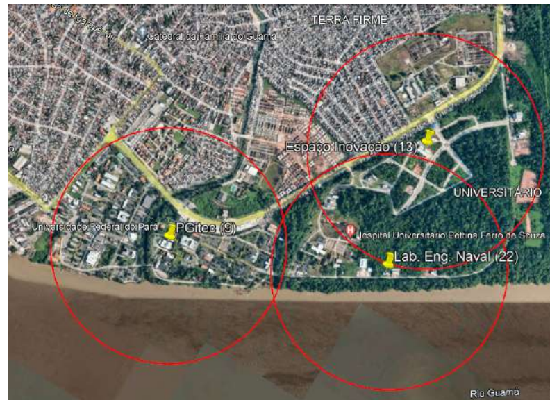
Figure 13. Optimal gateway placement for sensitivity of -108 dBm.
