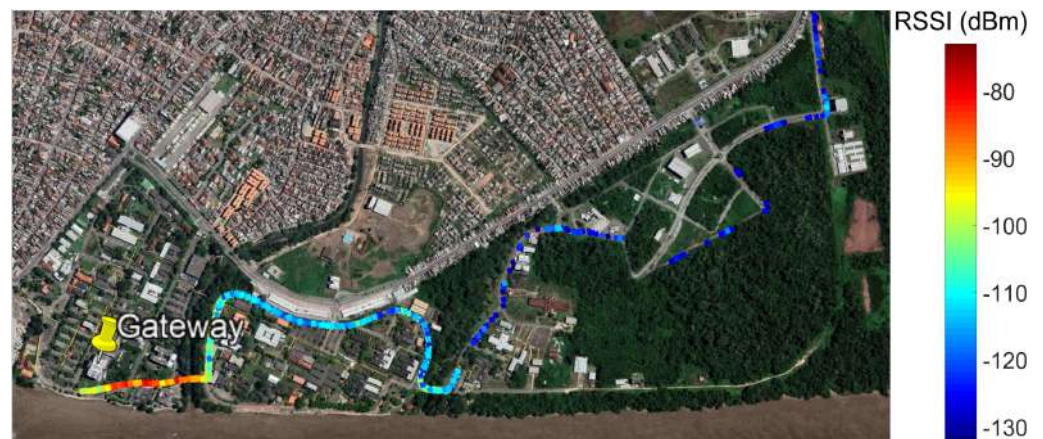
Figure 8. Route with measured data with location and RSSI value.
